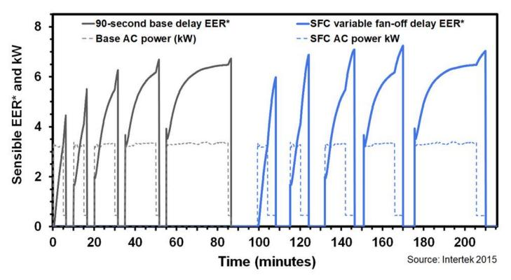
SFC variable cooling fan-off delay versus 90-second base delay for 3-ton unit
