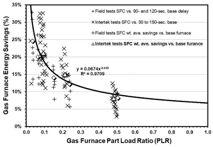
Gas Furnace Energy Savings as a Function of Part Load Ratio (PLR)
