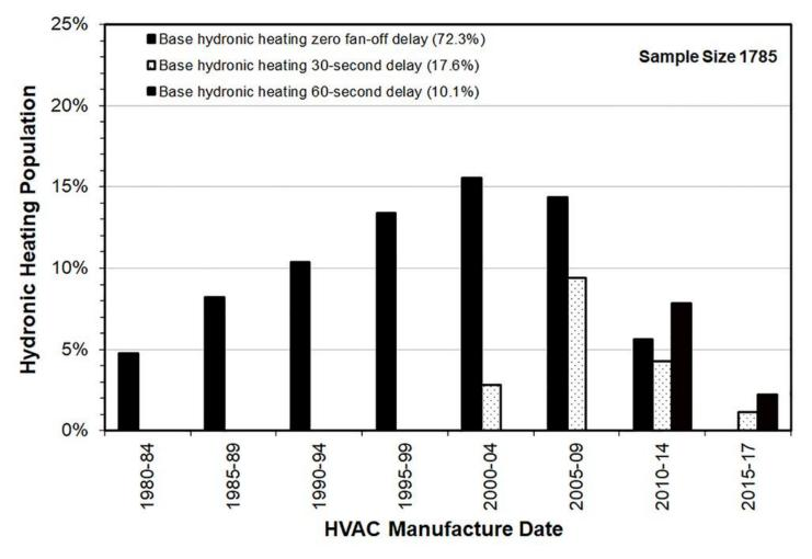
Distribution of Hydronic Heating Equipment Age and Base Heating Fan-Off Delay
