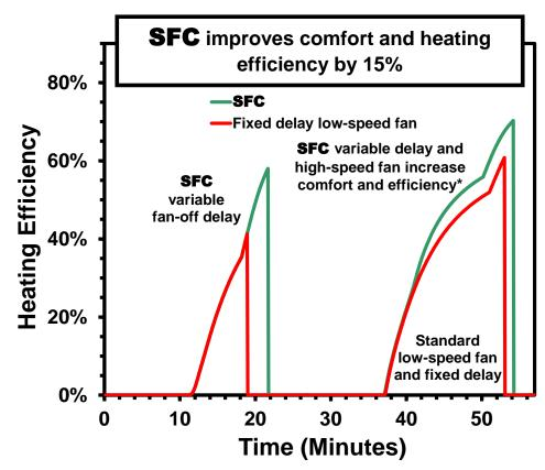
\*SFC high-speed fan saves gas by satisfying thermostat call for heating (right green curve) before standard low-speed fan (red curve).
