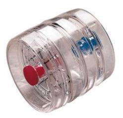
*Figure 2: Sensidyne 37mm directionnel air flow semple cassette.*
