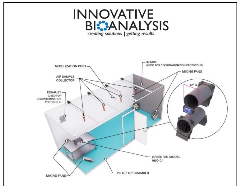
*Figure 4. Testing layout for control and experimental trials. Testing chambers exhaust and intake are not used during active virus testing outside of the decontamination function.*
